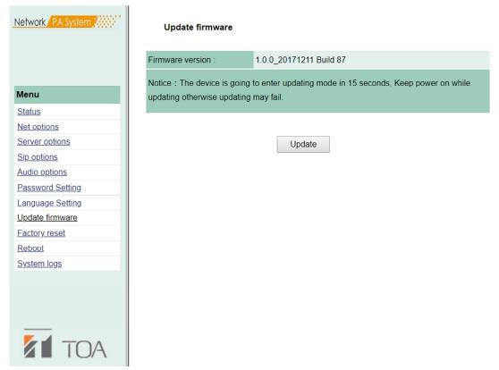
Note: Do not turn off the power during upgrading the terminal, otherwise it may lead to the failure of the upgrade and the failure of the equipment.
