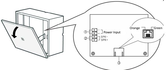
(1) Power Input connector: DC24V/1A is required, power supply input for network wall speaker. (Note: This equipment supports POE power supply. If the network interface is connected to POE switch, no power supply is needed)
